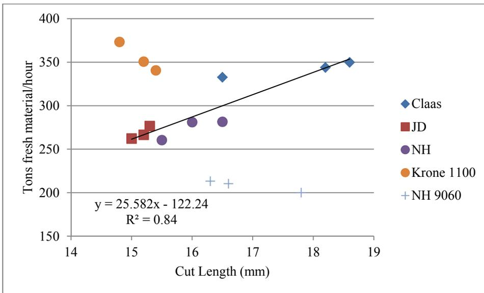
Figure 2. Tons Fresh Weight per Hour Chop Time Cut versus Length (2012).
