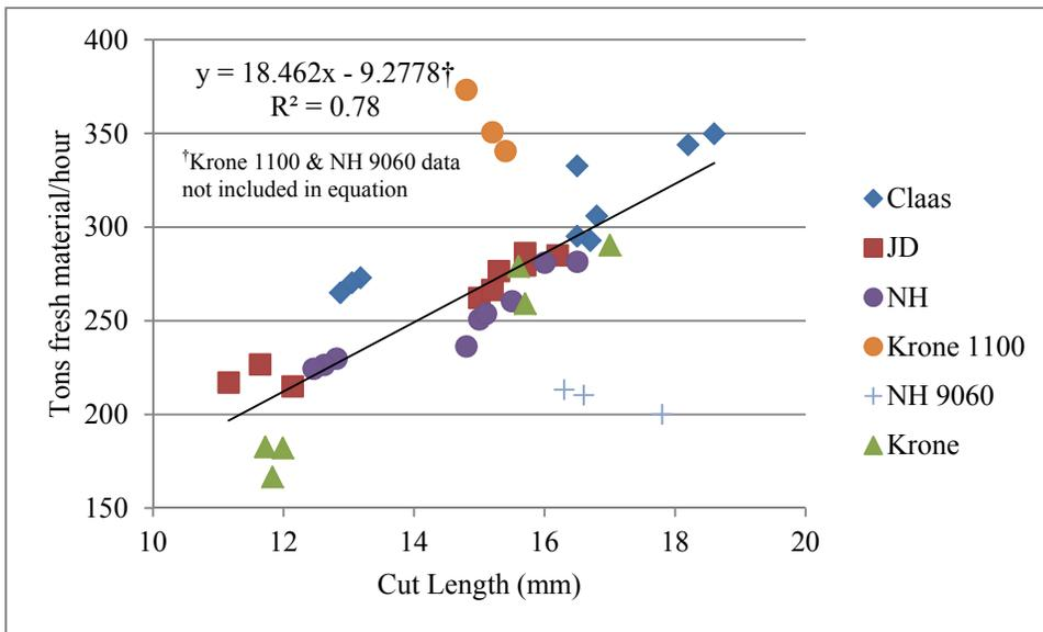
Figure 3. Tons Fresh Weight per Hour Chop Time versus Cut Length (2010-12).
