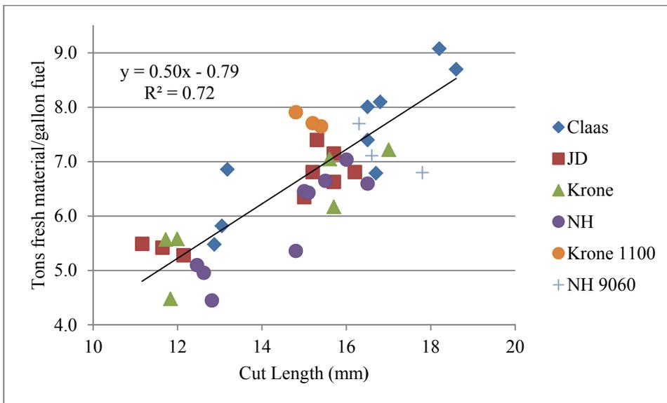
Figure 4. Tons Fresh Weight per Gallon of Fuel versus Cut Length (2010-12).
