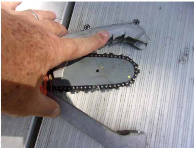
A chain-pole-saw allows an operator to cut overhead branches—with caution! Below is a battery-powered chain saw that can be used with a short pole or a longer pole using all three segments. A major disadvantage of this unit is that it does not have an automatic chain oiler. The unit comes with a squirt bottle to be filled with oil and applied to the chain at regular intervals.
