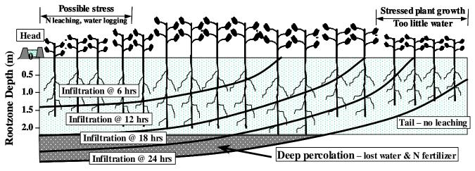
Fig. 4. Cross-section of crop rootzone during a 24 hour furrow irrigation.
