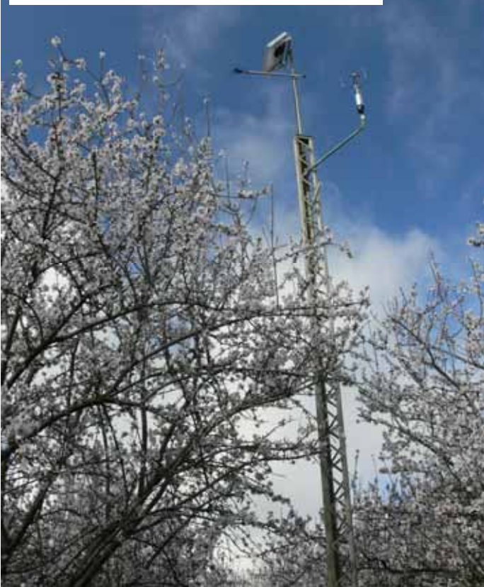
Sonic anemometer/eddy covariance tower for measuring almond ET
